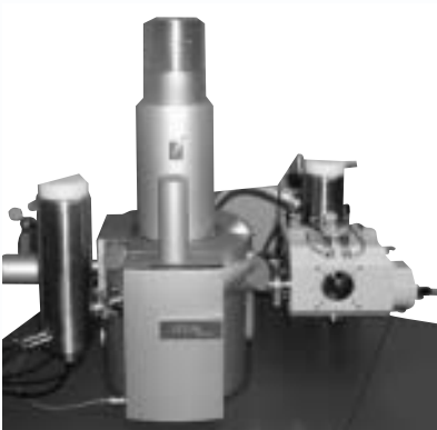
Tescan SEM with Cryo-SEM preparation system by Quorum Technologies.
