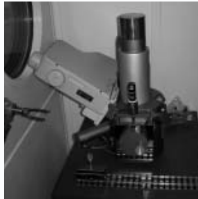
Remote controlled Tescan VEGA SEM placed in a "Hot Cell"
